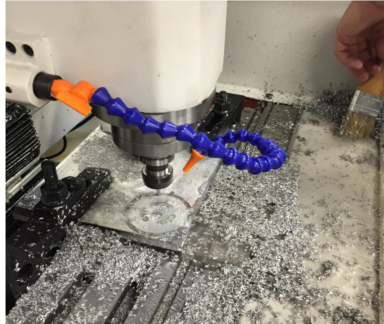
Cutting Gear Profiles on Tormach CNC Mill
